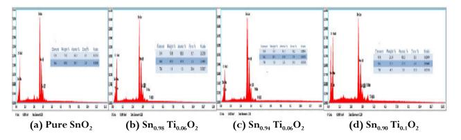
Fig. 3: EDAX images of pure and titanium doped tin oxide
