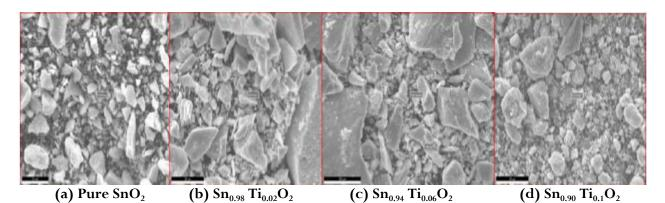
Fig. 2: SEM images of pure and titanium doped tin oxide
